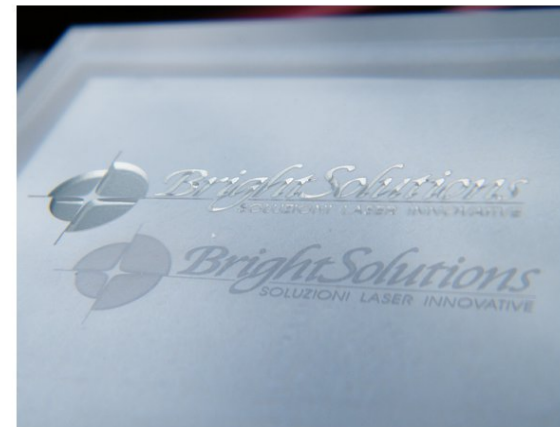
Surface engraving on glass
