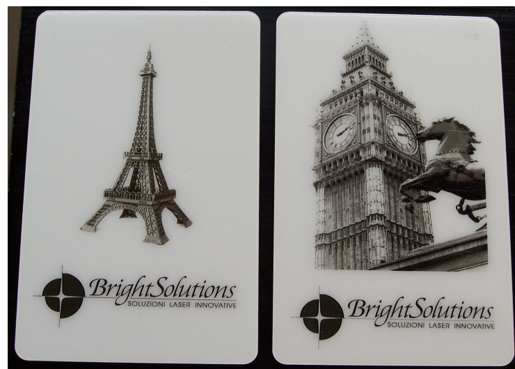
Grey Scale Images obtained using Pulse Energy Modulation
